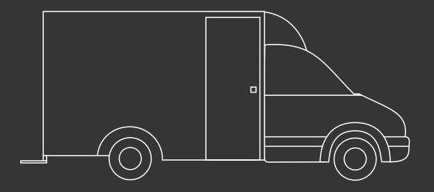
INTEGRAL WALK-IN BODY FOR VAN CHASSIS FROM 3.5 T TO 5.0 T
