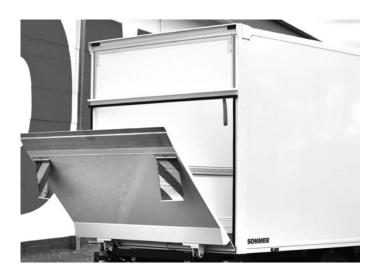
We can also supply the **SOMMER TG** on request with suitable ready-to-use tail-lifts. We offer a choice of various models from the most important suppliers with load capacities of 750 kg or 1,000 kg.
