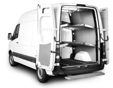
Thanks to its optimum utilization of space, the SOM-MER TA panel van shelf conversion provides generous storage possibilities not only in the shelves themselves but also for bulk items. A robust design with a 200 kg loading capacity per shelf and a stable partition wall along with a lockable sliding door are a matter of course with SOMMER.
